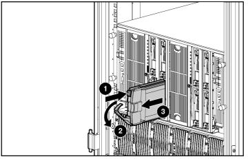
Figure 1-24: Removing a hot-plug SCSI hard drive
